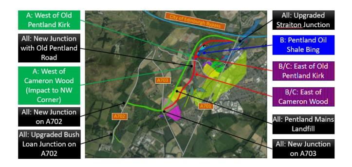
3.3 Route Options D, E, and F, are presented in the image below. The A702 Link Road section is the same for all of these option, beginning with a new at-grade 4-arm roundabout at the Bush Loan junction on the A702. It then continues east to a new at-grade 4-arm roundabout on the A703 – in the vicinity of Seafield Mill.
